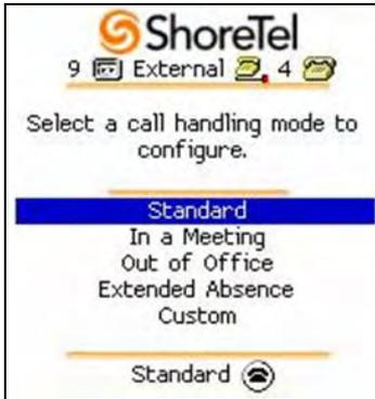
Scroll to the desired Call Handling Mode and press the track wheel to select it.
