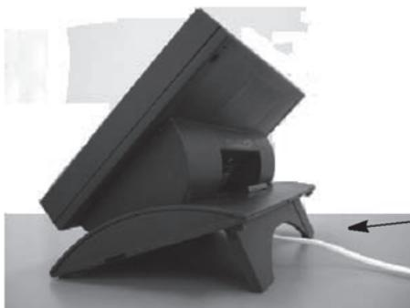
When the tilt stand extension is used, simply remove the line cord from under the rear cable clip. This will allow the tilt stand extension to deploy without strain on the line cord.
